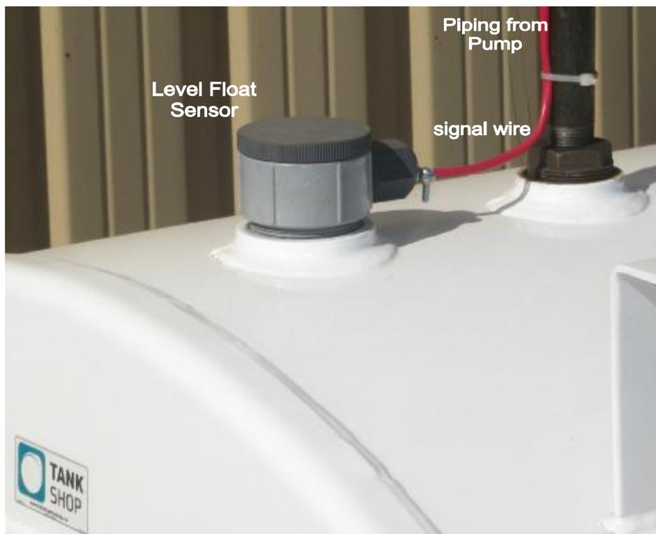
9. **Connect 1" piping** between storage tank and air diaphragm pump (top 1" port). This piping is not supplied with remote pump. Metal piping (ex.: steel) is preferred. The use of plastic piping is not recommended because of the ease of breaking down leading to leaks.
